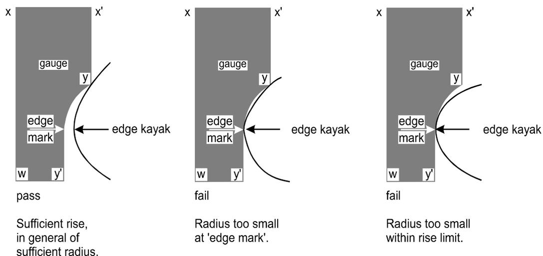
2.3. To gauge the radius of curvature the radius portion of the appropriate gauge, must be applied perpendicular to the surface being tested. If both points X and X' touch the surface at the
